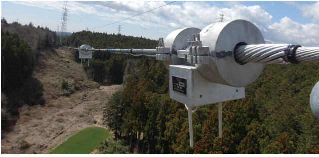
Photo 1. Appearance of transmission line sensor
