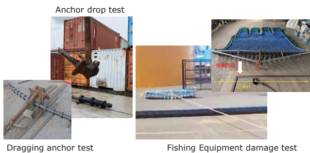
Photo 3. Cable damage test by anchor / bottom trawl tool
