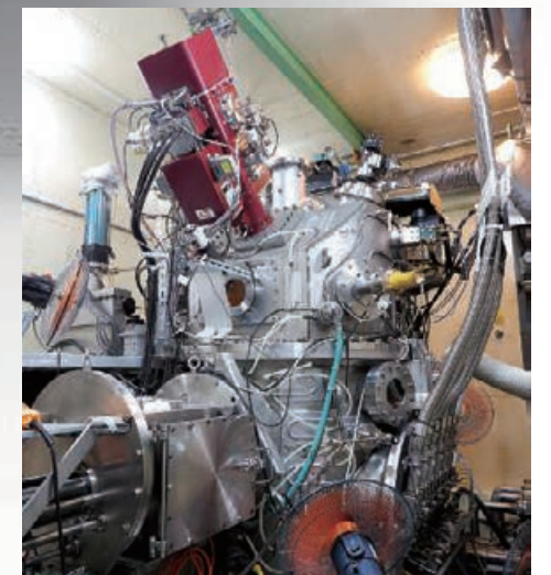
High heat flux test equipment (JEBIS) ©QST
