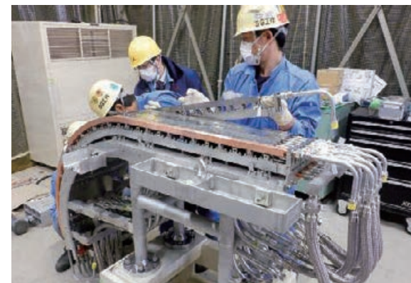
Installing monoblocks in the outer vertical target ©QST
