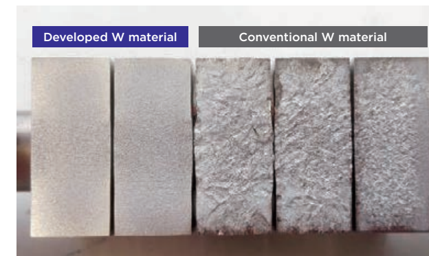
Tungsten monoblocks after high heat flux tests ©QST
