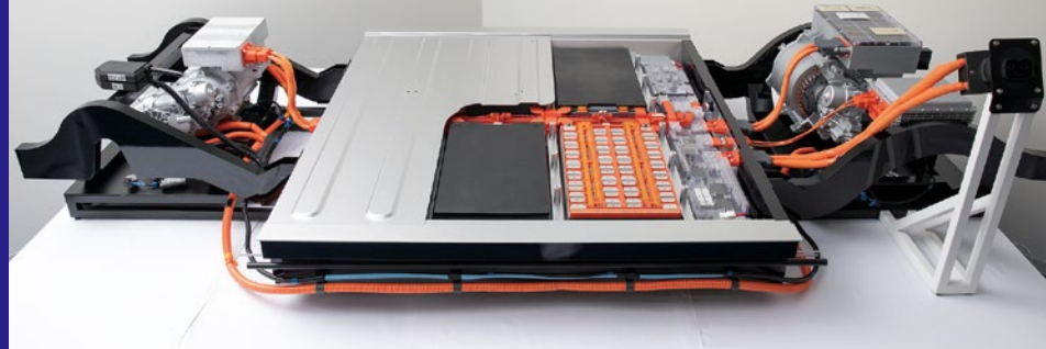
Battery bus bar module (BBM)
