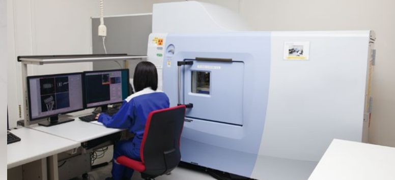
A micro-focus X-ray CT scanner uses X-rays to perform nondestructive three-dimensional observation of the internal structure of a specimen.
