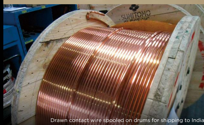
Drawn contact wire spooled on drums for shipping to India
