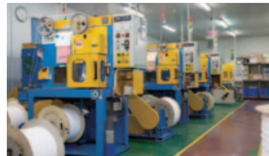
Top-Bottom) Hollow fiber membrane processing equipment operating in the factory
