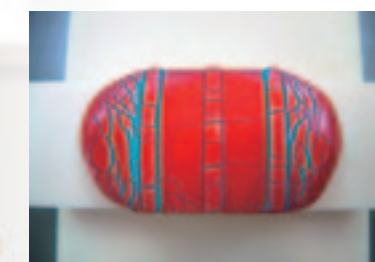
When a mock clay wire is compressed with a simulation terminal, significant deformation and breakage of the painting layer occur in the vicinity of the serration.
