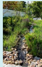
A "waterscape," which creates a natural river using circulated rainwater
