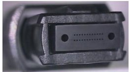
Connector terminal (ferrule) cross-section
