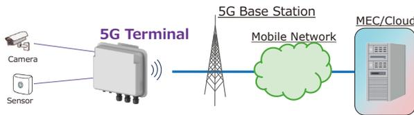
Fig. 13. Appearance of 5G millimeter-wave terminal and example system configuration
