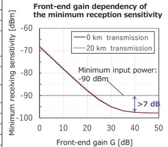
Fig. 7. Frontend gain dependency of unlink A-RoF uplink reception
