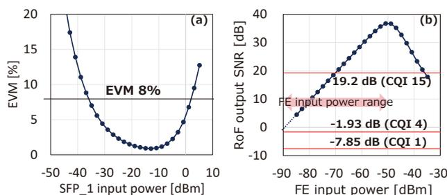
Fig. 11. (a) EVM measurement result, (b) estimated SNR of RoF output signal
