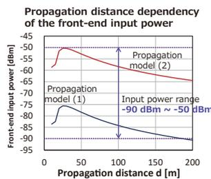
Fig. 6. Uplink input power range at Front End
