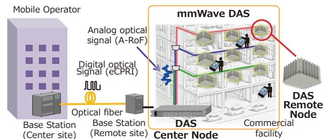
Fig. 12. Millimeter-wave distributed antenna system
