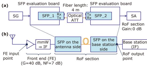
Fig. 10. (a) Evaluation setup of transmission characteristics for the SFP-type A-RoF optical module, (b) corresponded base station uplink architecture
