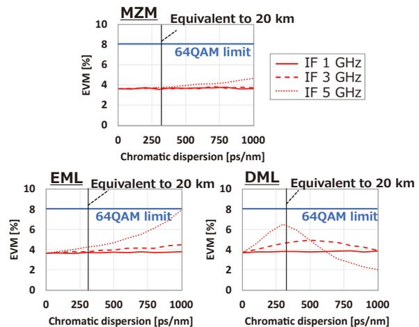
Fig. 4. Influence of chromatic dispersion caused by standard single mode fiber transmission
