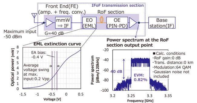
Fig. 8. Signal spectrum after A-RoF transmission when Front End input signal power is maximum
