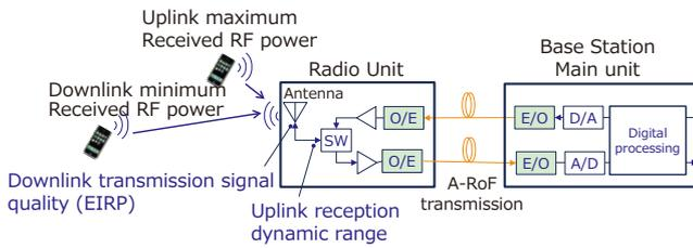
Fig. 2. Downlink transmission signal quality and uplink reception dynamic range
