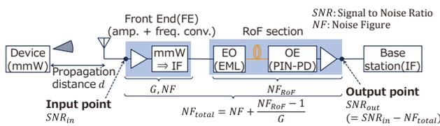
Fig. 5. Block diagram of uplink A-RoF reception
