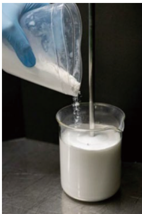
Photo 1. Silica aerogel transformed into paint
