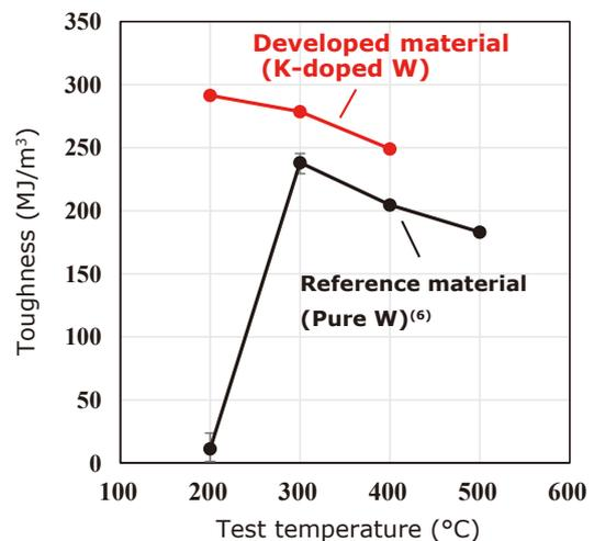
Fig. 5. Relationship between test temperature and the toughness of material after heat treatment
