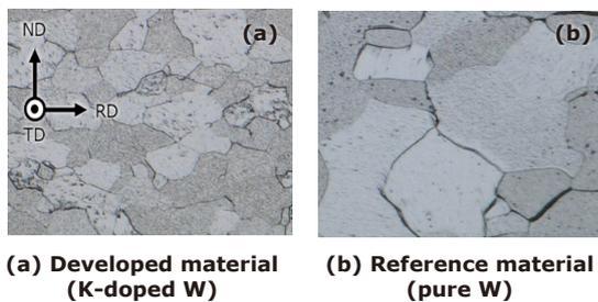
Fig. 4. Microstructure of materials after heat treatment
