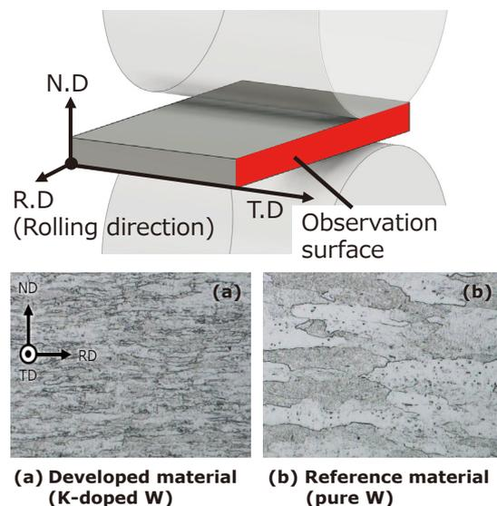
Fig. 3. Microstructure of materials as manufactured
