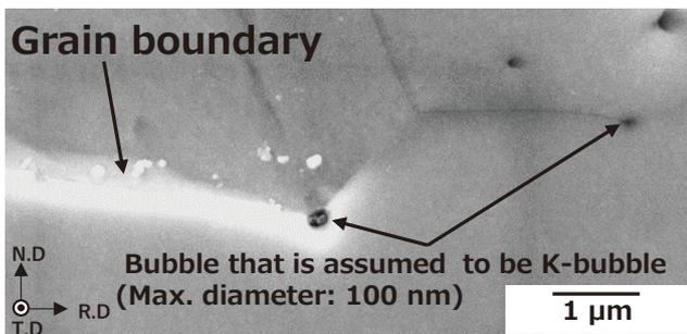
Photo 2. Scanning electron micrograph of material after heat-treatment
