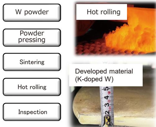
Fig. 1. W material manufacturing method
