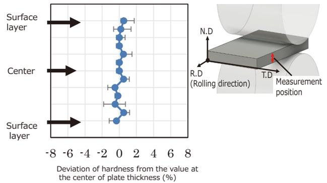
Fig. 2. Deviation of hardness of developed material in the thickness direction of TD cross section
