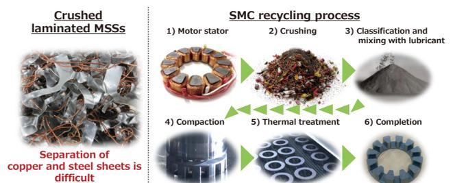
Fig. 5. Targeted SMC recycling process
