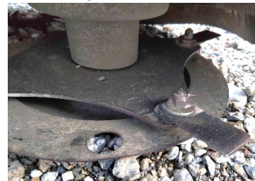
Standard cutting blade appurtenant to the grass trimming attachment
