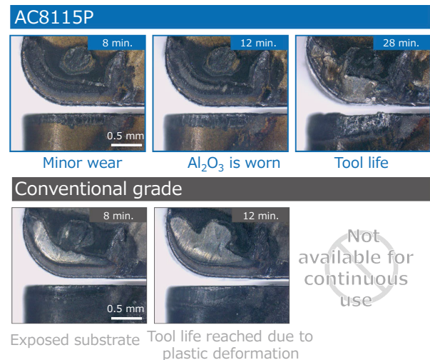
Fig. 7. Comparison of damage conditions at v_c = 350 m/min
