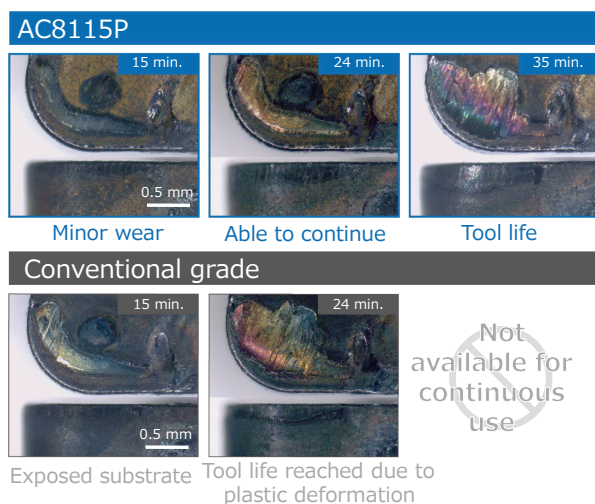
Fig. 10. Comparison of damage in dry cutting
