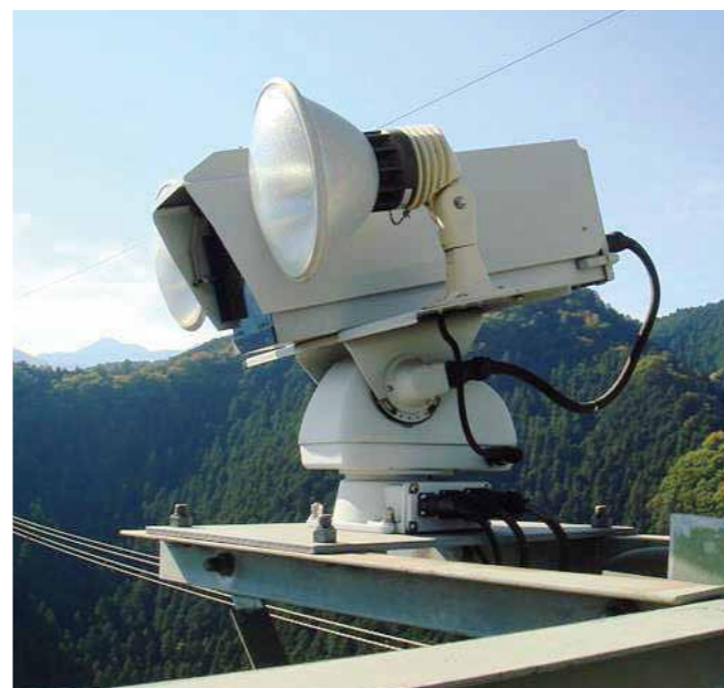
Controllable camera for monitoring overhead lines
