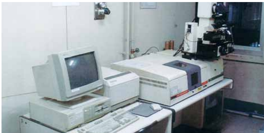
FTIR (Fourier Transform Infrared Spectroscopy) Analysis System, to investigate the new insulation material
