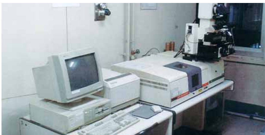
FTIR (Fourier Transform Infrared Spectroscopy) Analysis System, to investigate the new insulation material
