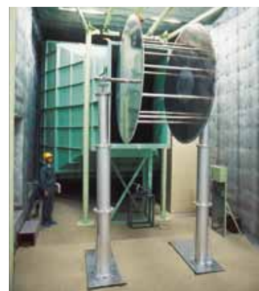
Wind tunnel facility to develop Aeolian noise suppressed conductor
