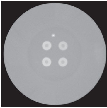
Photo 1. A cross section of a fabricated C-MCF (7)
