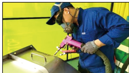
Photo 2. Utilization of fiber laser welding
