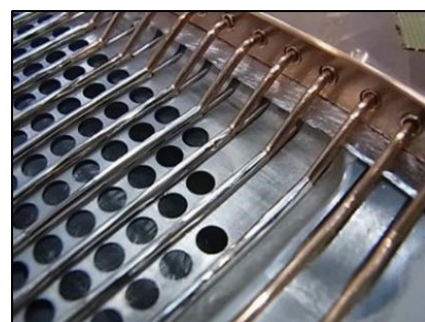
Photo 9. Example of simultaneous, airtight vacuum brazing of multiple points
