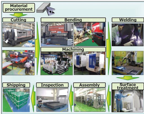
Fig. 2. Integrated manufacturing system
