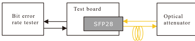
Fig. 8. Receiver characteristics test system
