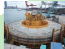
Extra high voltage DC cable
