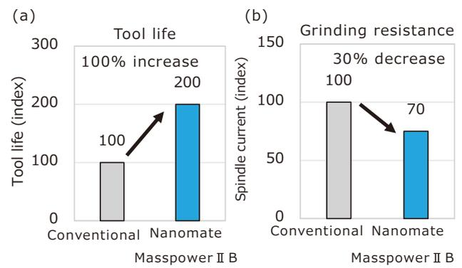
Fig. 2. 8-inch SiC wafer processing examples: (a) tool life and (b) grinding resistance
