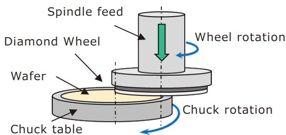
Fig. 1. Vertical rotary surface grinding
