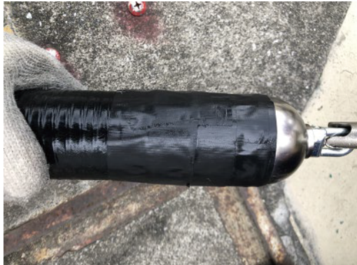
Photo 2. Appearance of the protection sleeve for a pre-connectorized small-diameter 3456-fiber-count cable after a durability test
