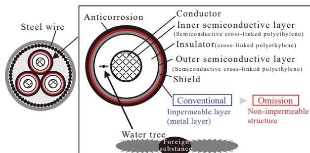
Fig. 1. Non-impermeable submarine cable and water tree
