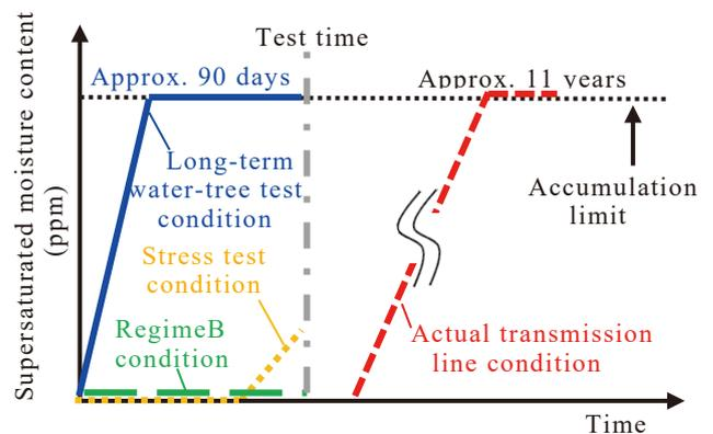
Fig. 6. Time for supersaturated moisture to reach the accumulation limit
