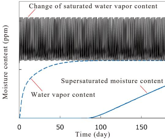
Fig. 5. Supersaturated moisture content of insulator’s middle and inner layers (stress test)
