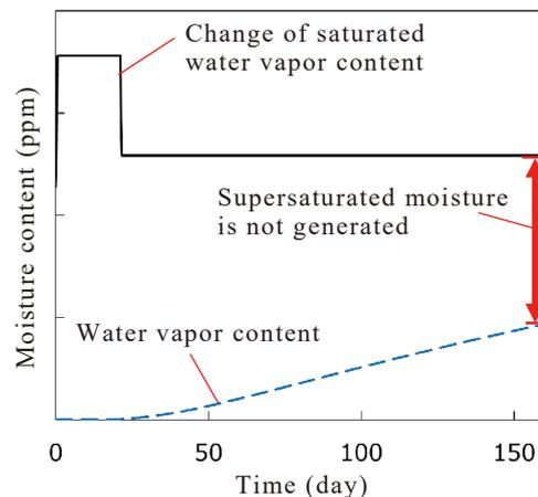
Fig. 4. Supersaturated moisture content of insulator’s inner layer: CIGRE TB722 RegimeB
