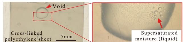
Photo 1. Supersaturated moisture generated in a void in a cross-linked polyethylene sheet
