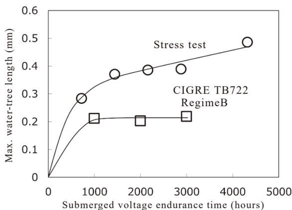
Fig. 2. Relationship between submerged voltage endurance test condition and maximum growth length of water tree
