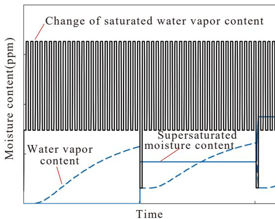
Fig. 3. Supersaturated moisture content of insulator’s inner layer: actual transmission line condition
