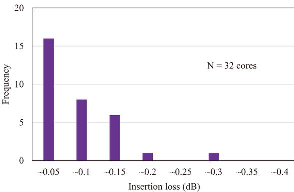
Fig. 6. IL estimates calculated from bundle core eccentricity
