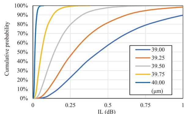
Fig. 4. IL yield rate by fiber diameter
