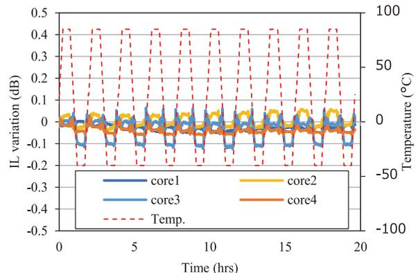
Fig. 13. Temperature-dependent loss
