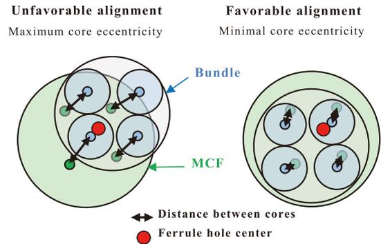
Fig. 7. Schematic diagram of a rotational alignment
