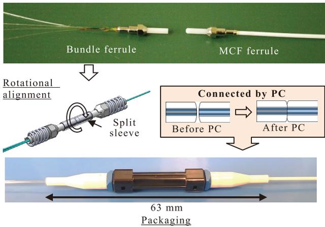
Fig. 2. FO device assembly and PC connection
