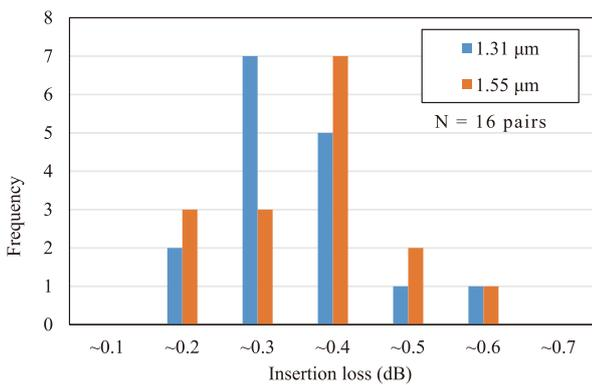
Fig. 10. IL measurement result
