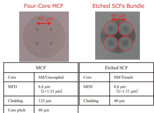
Fig. 1. Specifications of 4-core MCF and bundle
