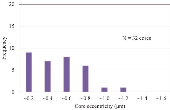
Fig. 5. Core eccentricity of the fabricated bundles measurement
