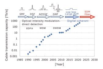
Fig. 2. Cable transmission capacity and optical fiber technology
