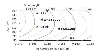
Fig. 3. Span length as a function of A<sub>eff</sub> and transmission loss (Transmission distance: 7,000 km, 48 cores, Cable transmission capacity: 0.5 Pb/s)
