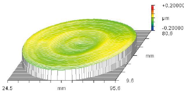
Fig. 7. Figure accuracy of aspheric surface
