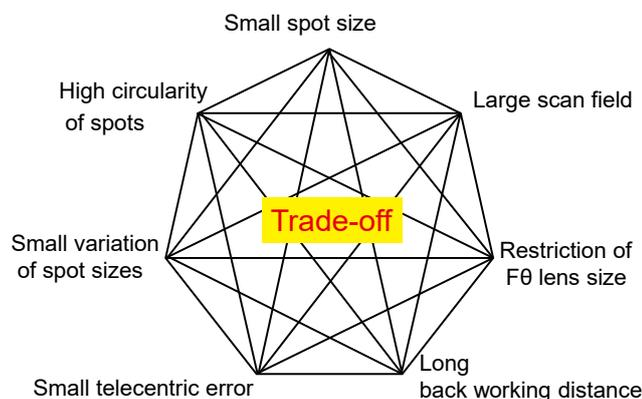
Fig. 2. Schematic diagram showing trade-off relationship of characteristics for F $\theta$  lens
