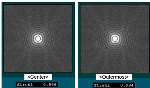
Fig. 10. PSF (center and outermost positions of scan field)
