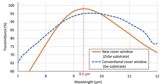
Fig. 8. Measured transmission spectrum of cover window
