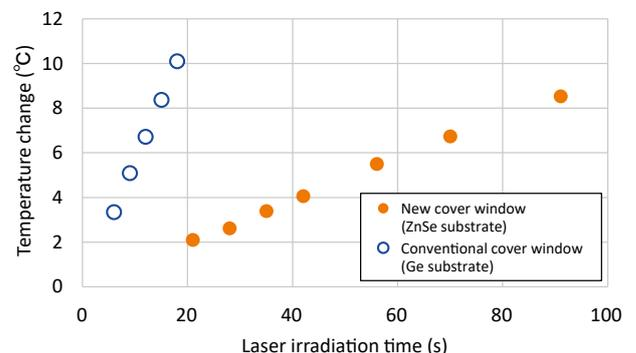
Fig. 9. Temperature change of cover window irradiated with a CO<sub>2</sub> laser
