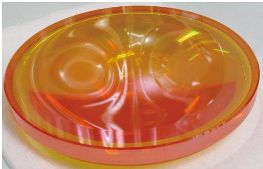
Photo 1. Aspheric lens having a large sag difference
