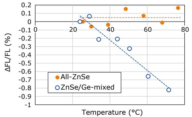
Fig. 11. Temperature dependence of focal length (FL)
