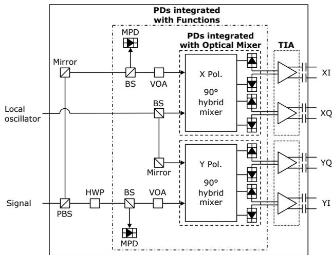
Fig. 1. Internal structure of coherent receiver
