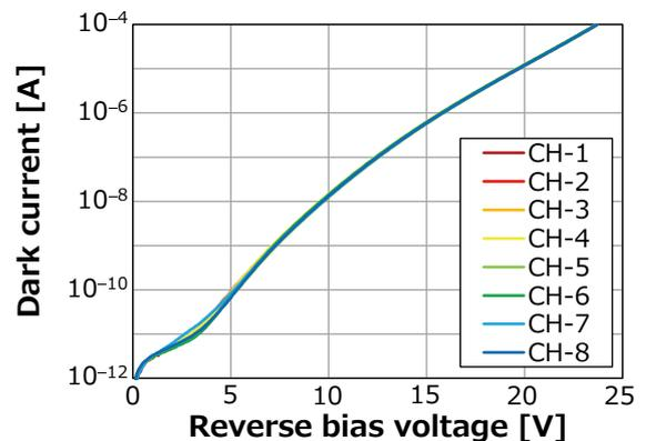
Fig. 7. Reverse bias I-V characteristics of multifunctional integrated photodetector
