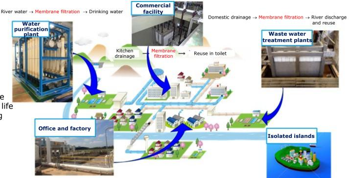
Factory wastewater  $\rightarrow$  Membrane filtration  $\rightarrow$  River discharge and reuse
