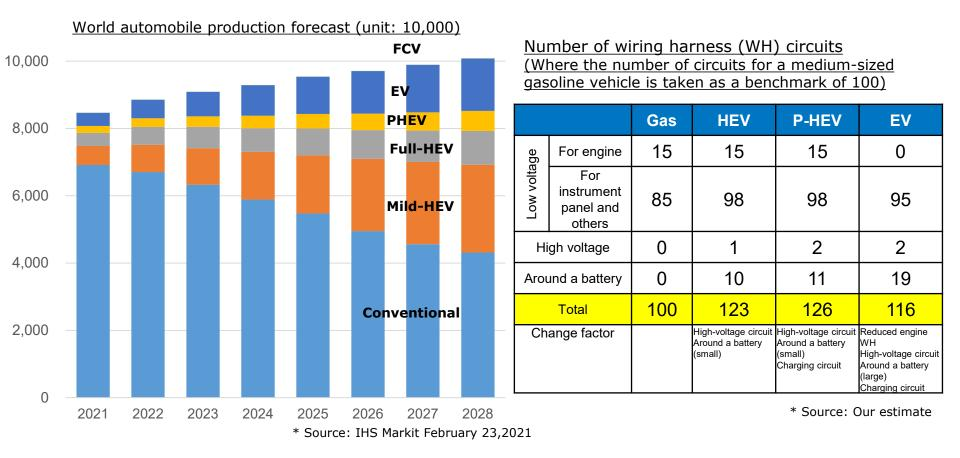
The shift to xEVs increases the number of wiring harnesses for high-voltage purpose and around a battery. (EVs do not require a wiring harness for an engine.) ⇒ <u>Overall, the number of circuits</u> increases, particularly due to the increasing demand for wiring harnesses around a battery.
