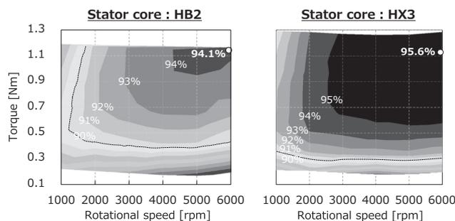
Fig. 3. Efficiency maps of newly developed AGMs
