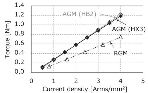
Fig. 4. Torque characteristics of newly developed AGMs
