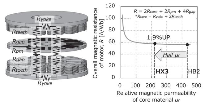
Fig. 5. Magnetic resistance of AGM vs. magnetic permeability of core
