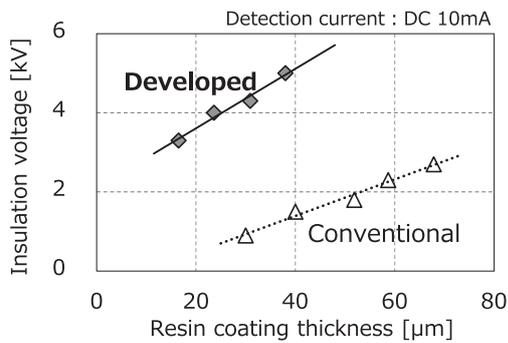
Fig. 6. Insulation voltage of the newly developed coating
