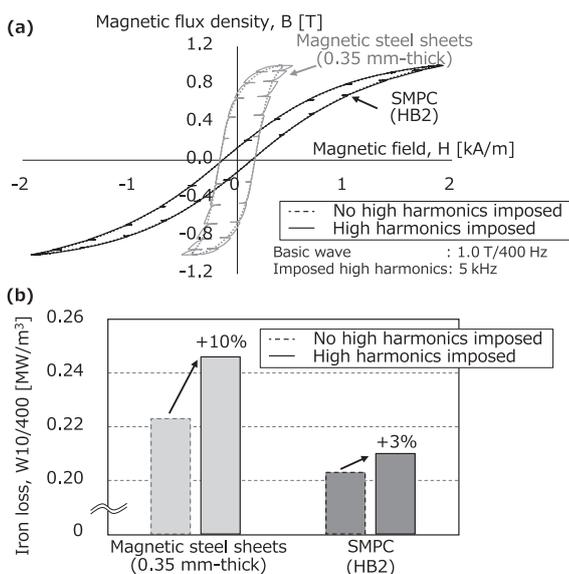
Fig. 1. Differences in hysteresis loop (a) and iron loss (b) with high harmonics imposed and not imposed
