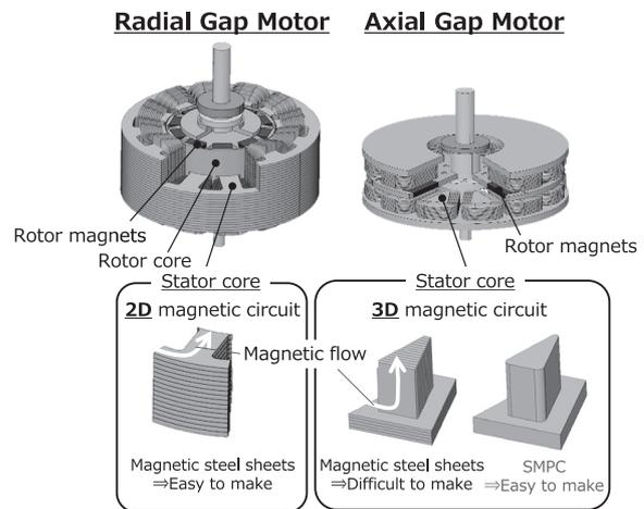
Fig. 2. Different motor structures
