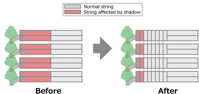
Fig. 11. Example of proposal on string rewiring work
