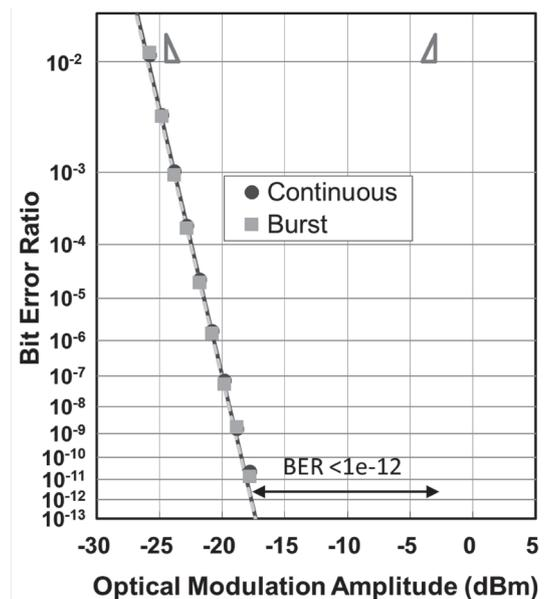
Fig. 7. 25.78 Gbit/s Bit Error Ratio results
