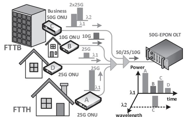
Fig. 1. 50G-EPON system overview and upstream transmission
