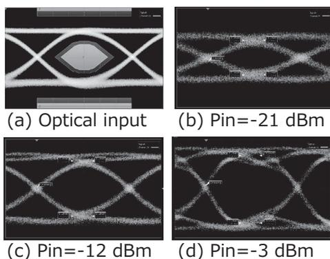
Fig. 5. 25.78 Gbit/s optical input and electrical output waveforms
