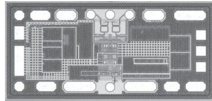
Photo 2. A photo of BM-TIA IC chip
