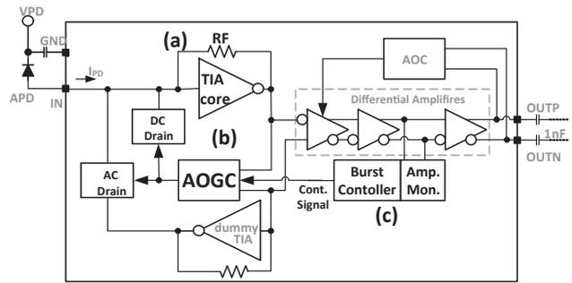
Fig. 2. Block diagram of 25.78 Gbit/s BM-TIA
