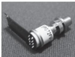
Photo 1. Burst-Mode receiver for 50G-EPON OLT
