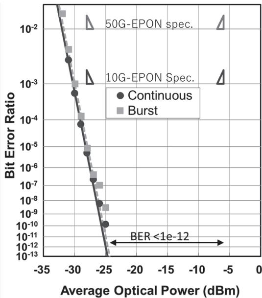
Fig. 8. 10.31 Gbit/s Bit Error Ratio results
