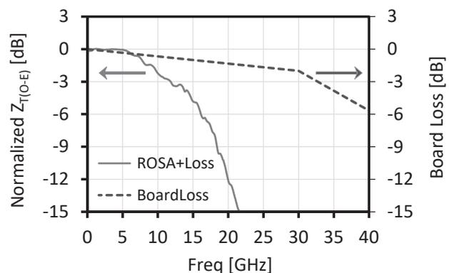
Fig. 3. High-frequency response of optoelectronic conversion gain ( $Z_{T(O-E)}$ )
