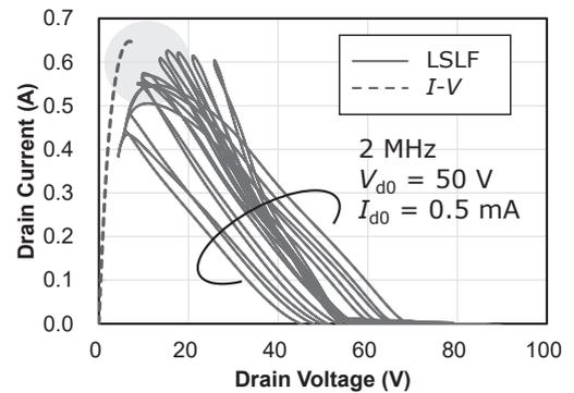
Fig. 6. Load lines obtained by LSLF measurements
