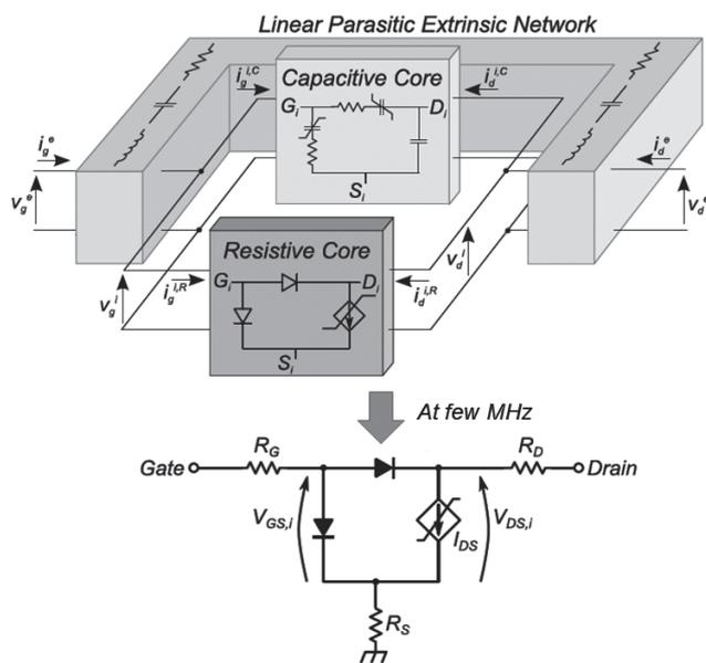
Fig. 5. Principle of LSLF measurements<sup>(9)</sup>
