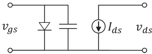
Fig. 8. Large-signal model of GaN HEMT
