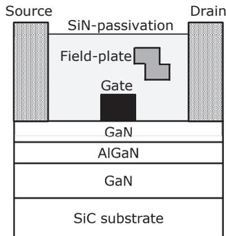
Fig. 2. Schematic cross-sectional structure of GaN HEMT
