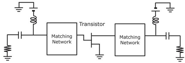
Fig. 3. Simplified equivalent circuit of a GaN HEMT amplifier
