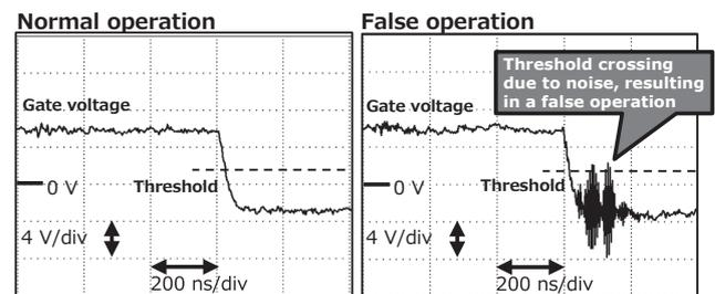
Fig. 4. False operation waveforms of GaN device
