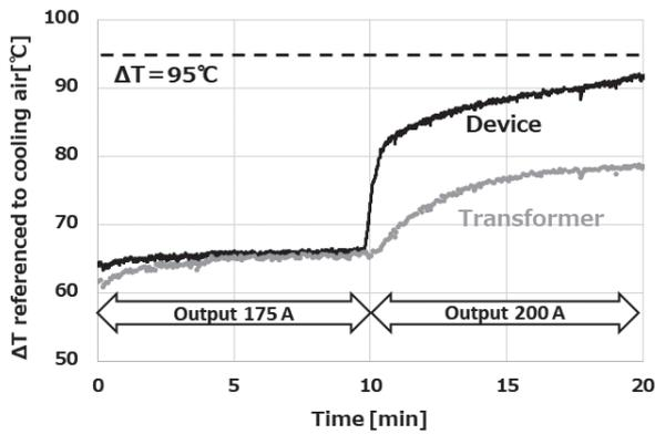
Fig. 9. Temperature increases in principal heat-generating components
