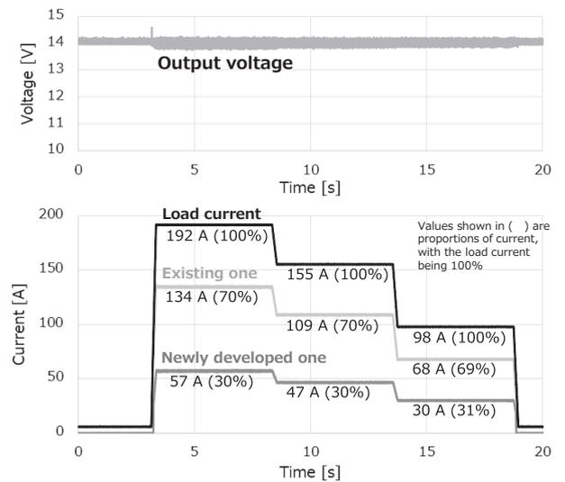
Fig. 14. Verification of actual converters in parallel operation
