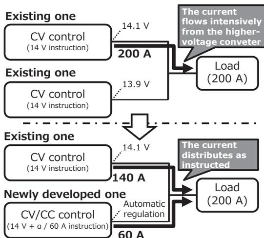
Fig. 13. Parallel converter operations
