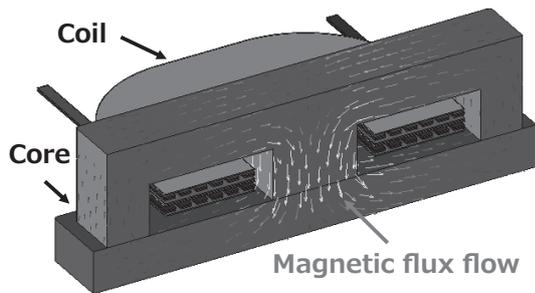
Fig. 6. Analyzed magnetic flux flow of transformer
