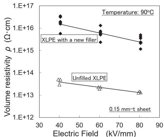
Fig. 8. Electric field dependence of volume resistivity of XLPE with a new filler (DC-XLPE) and unfilled XLPE (AC-XLPE)<sup>(17)</sup>
