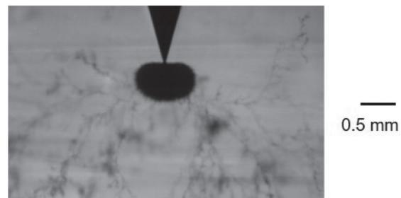
Photo 3. Feature of electrical trees (an Aegagropila-like tree & Cotton-like trees) after AC 18 kV  $\times$  30 min. & AC 10 kV  $\times$  2 h voltage application<sup>(4)</sup>
