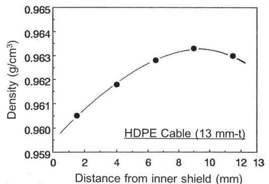
Fig. 5. Density distribution of HDPE cable insulation (13 mm-t)<sup>(13)</sup>
