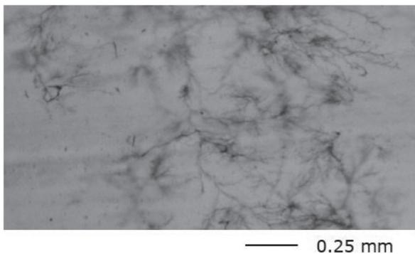
Photo 2. Electrical trees in random directions (named “Cotton-like trees”) observed near a breakdown path in XLPE base insulation of a product<sup>(1)</sup>
