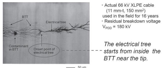
Photo 5. Example of electrical tree starting from a BTT in an actual 66 kV XLPE cable<sup>(22)</sup>
