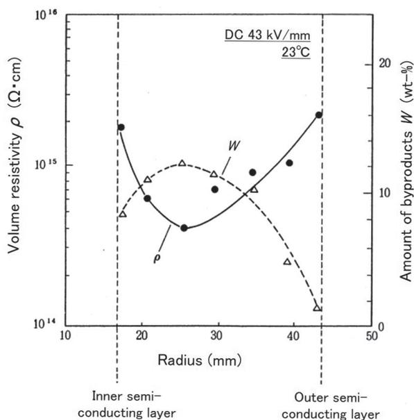
Fig. 2. Distribution of volume resistivity  $\rho$  and amount of peroxide byproducts  $W$  in 275 kV XLPE cable (27 mm-t, 600 mm<sup>2</sup>) in the radial direction of the insulator<sup>(12)</sup>
