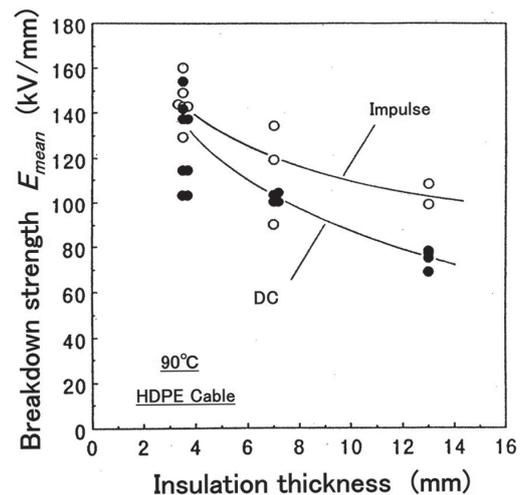
Fig. 4. Insulation thickness dependence of breakdown strengths of HDPE cables<sup>(13)</sup>
