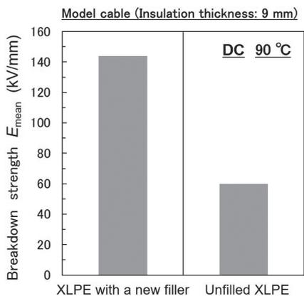
Fig. 10. DC breakdown strength of new XLPE cable with a new filler (DC-XLPE) and unfilled XLPE cable (AC-XLPE)<sup>(17)</sup>
