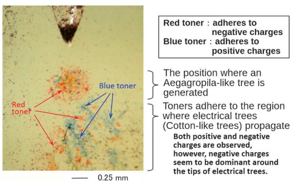
Photo 4. Dust figure pattern of treeing sample after AC 18 kV × 30 min. & AC 10 kV × 2 h voltage application<sup>(4)</sup>
