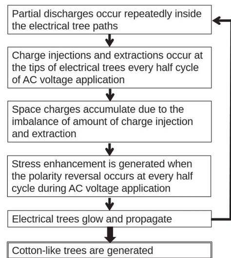
Fig. 1. Schematic representation of generation mechanism of Cotton-like trees<sup>(4)</sup>
