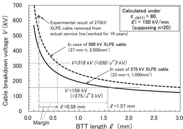
Fig. 14. Relationship between BTT length and breakdown voltage of 275 kV & 500 kV XLPE cables<sup>(23)</sup>
