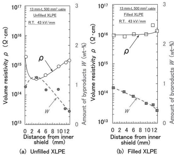
Fig. 6. Difference between filled and unfilled XLPE cables in volume resistivity  $\rho$  and amount of peroxide byproducts  $W$  in the radial direction of the insulator<sup>(15)</sup>
