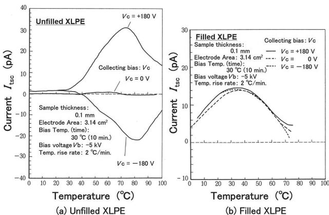
Fig. 7. TSC spectra of unfilled and filled XLPEs<sup>(15)</sup>
