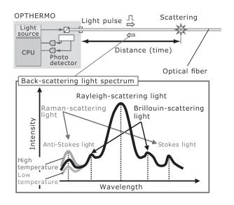
Fig. 1. OPTHERMO measurement mechanism
