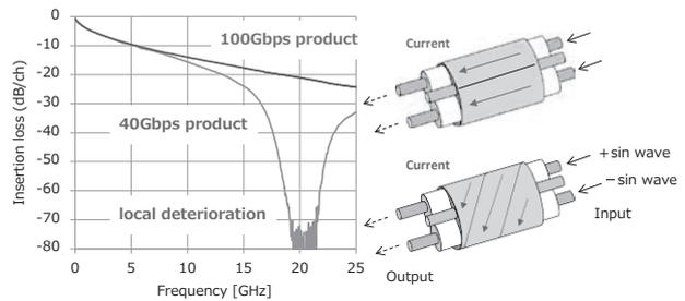
Fig. 2. Insertion loss waveform per channel
