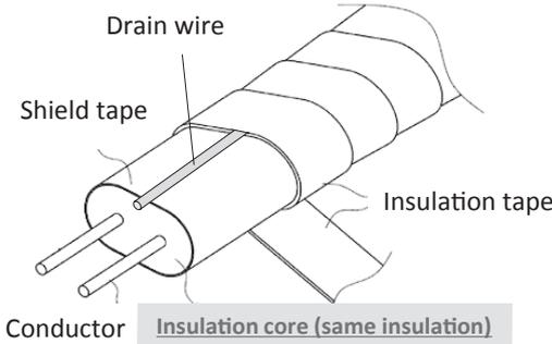
Fig. 5. Same insulation structure
