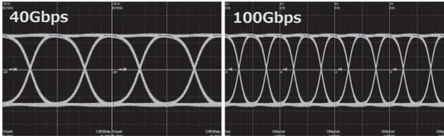
Fig. 3. Correlation between transmission speed and eye pattern
