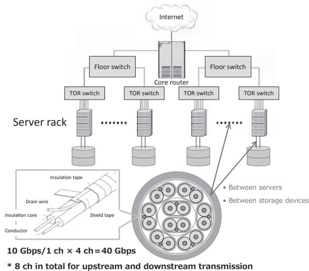
Fig. 1. Example of use at data centers
