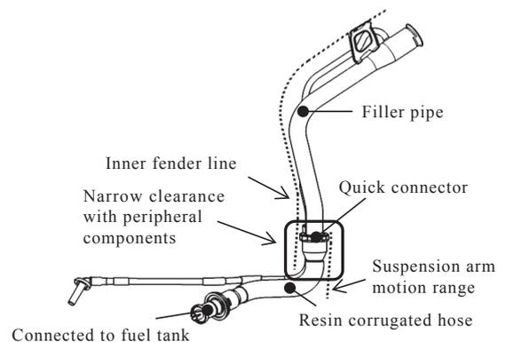
Fig. 6. Piping example using conventional resin filler hose
