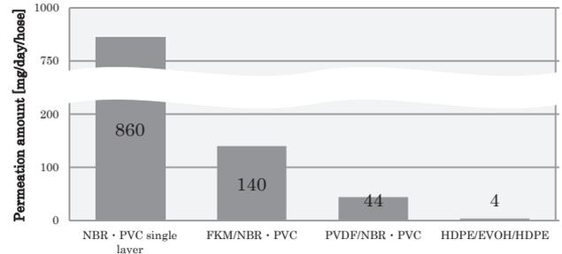
Fig. 5. Comparison between hose material configuration and fuel permeation amount
