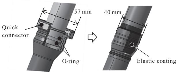
Fig. 7. Joining structure comparison with filler pipe
