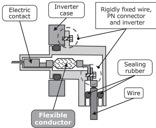
Fig. 3. Absorption of dimensional change of PN connector
