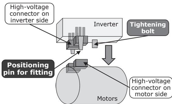
Fig. 5. Inverter and motors installing operation (First step)
