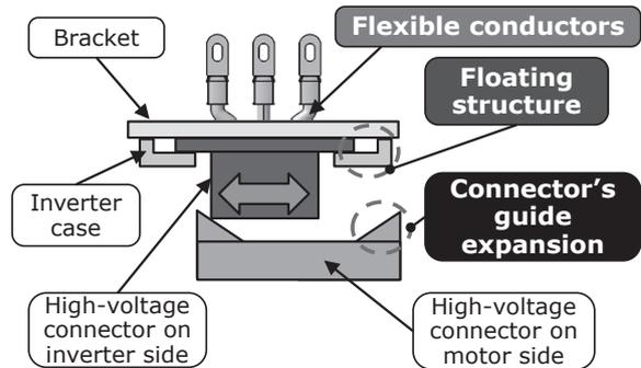
Fig. 6. High-voltage connector mating (Second step)
