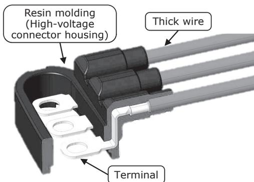
Fig. 4. Conceptual illustration of six-phase integral molding technique
