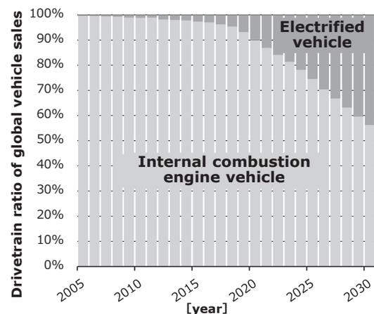
Fig. 1. Prediction of sales ratio of internal combustion engine vehicle and electrified vehicle
