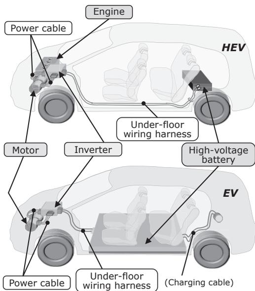
Fig. 2. Electric drivetrain of HEV and EV
