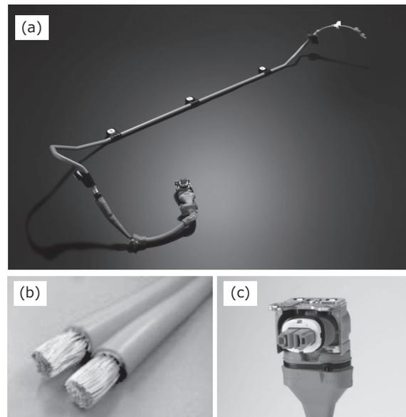
Photo 1. Pipe shielded wiring harness and PN connector
