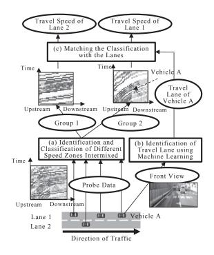
Fig. 3. System for generating lane-specific travel speed information
