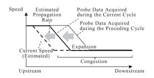
Fig. 4. Generation of travel speed information by estimating the propagation of traffic congestion
