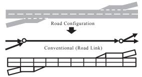
For autonomous vehicle (partition of each lane into small sections)
