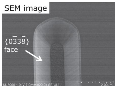
Fig. 3. SEM image of a formed trench
