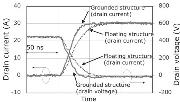
Fig. 6. Turn-on switching waveforms
