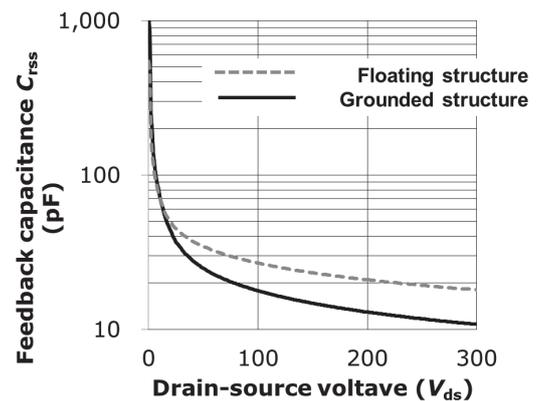
Fig. 4. Capacitance characteristics of SiC VMOSFET
