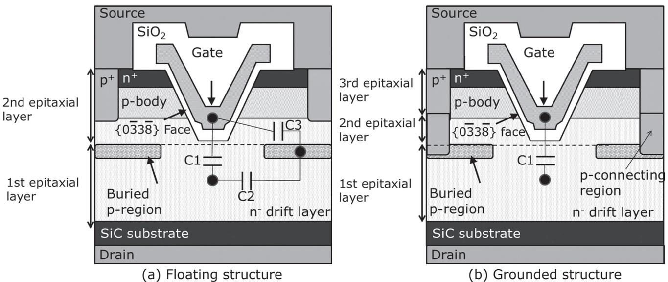
Fig. 1. Schematic cross-sectional diagram of SiC VMOSFET and  $C_{rss}$  components
