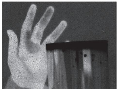
Photo 2. Thermal image of container cooled with liquid nitrogen
