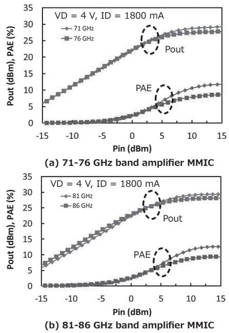
Fig. 8. Input-output power characteristics and PAE characteristics of the amplifier MMIC
