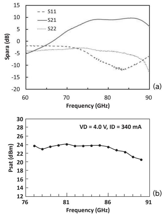
Fig. 5. Small signal characteristics (a) and saturated output characteristics (b) of the unit amplifier
