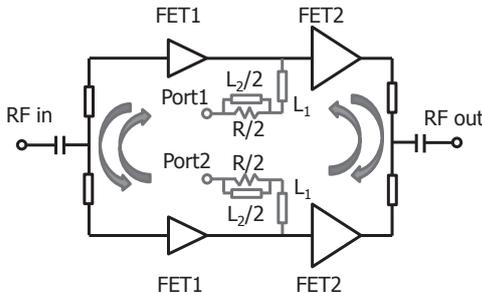
Fig. 3. Model simulating the stability of the unit amplifier
