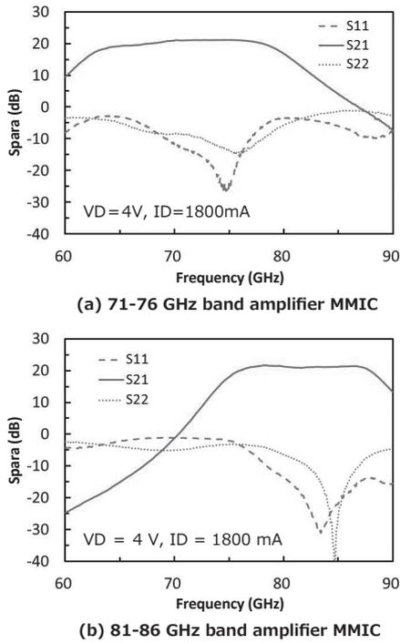
Fig. 7. Small signal characteristics of the amplifier MMIC
