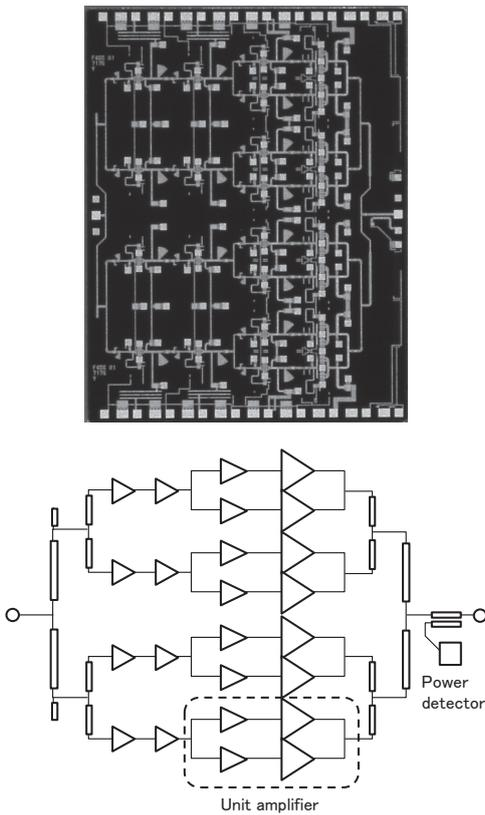
Fig. 6. Photo and block diagram of the amplifier MMIC
