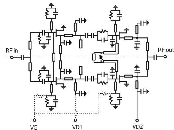
Fig. 2. Circuit diagram of the unit amplifiers
