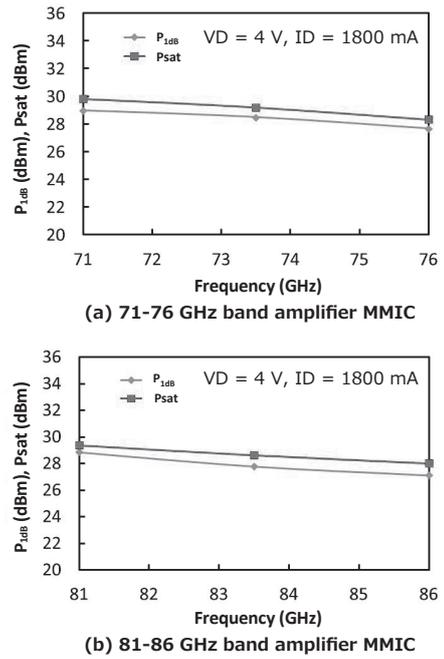
Fig. 9. Frequency characteristics of the P1dB and Psat of the amplifier
