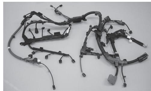
Photo 4. Engine wiring harness using high strength-aluminum wire
