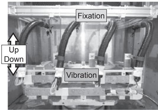
Photo 2. Situation of tests simulating engine vibration
