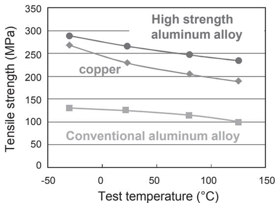
Fig. 7. Temperature characteristics of strength
