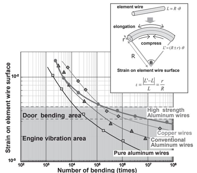
Fig. 5. S-N characteristics of various conductors
