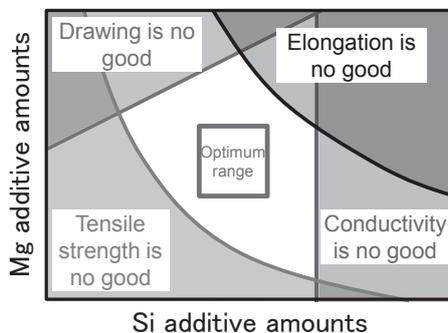
Fig. 2. Results of consideration of amount of Mg and Si addition
