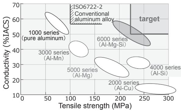
Fig. 1. Characteristics of various aluminum alloys
