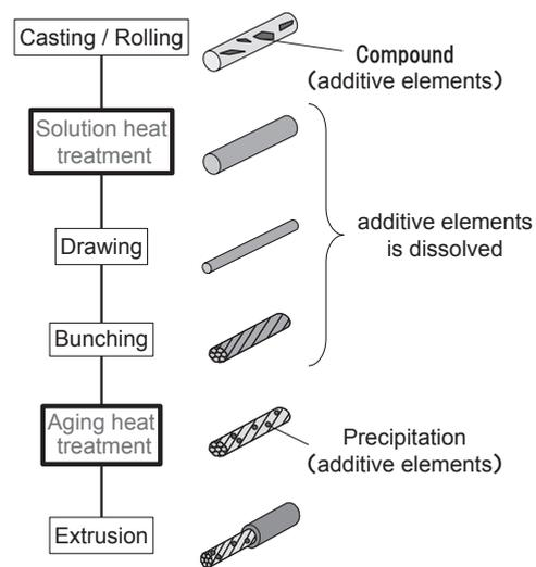
Fig. 3. Manufacturing processes for aluminum wire
