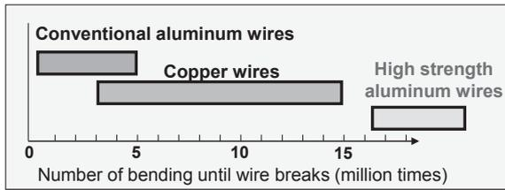
Fig. 6. Results of tests simulating engine vibration
