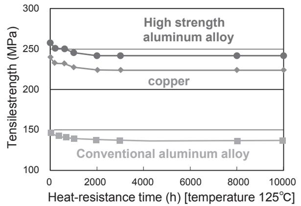
Fig. 8. Strength after high temperature storage
