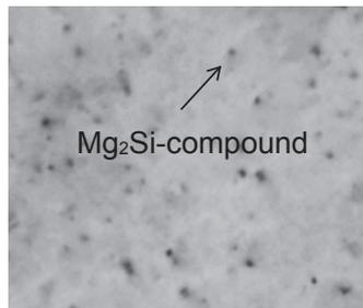
Photo 1. Finely dispersed Mg<sub>2</sub>Si intermetallic compounds
