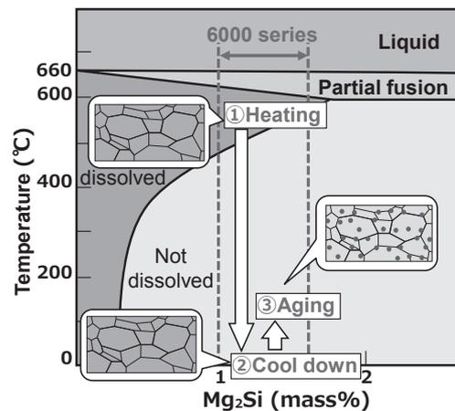
Fig. 4. Pseudo-binary phase diagram for Al-Mg<sub>2</sub>Si
