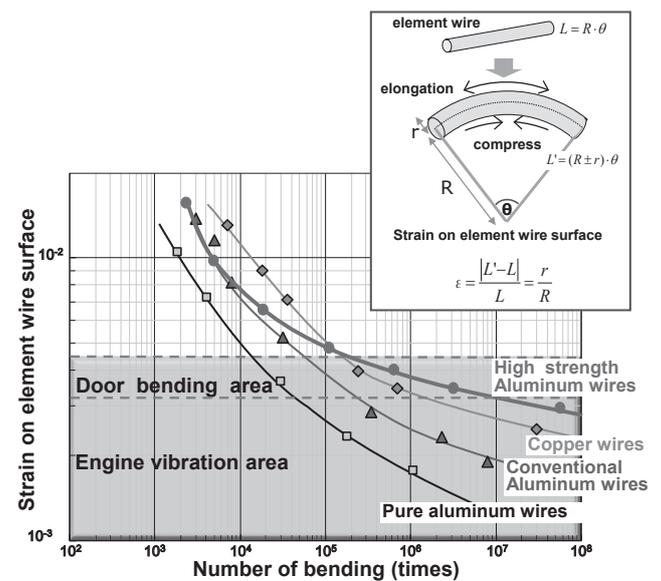
Fig. 5. S-N characteristics of various conductors
