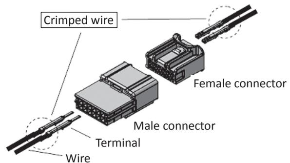
Fig. 9. Connectors and crimped wire
