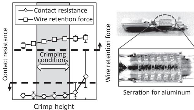
Fig. 11. Crimping characteristics of terminals for high-strength aluminum wires
