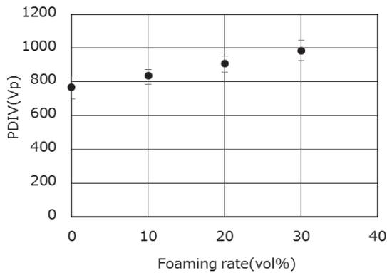
Fig. 7. PDIV Measurement Result for Magnet Wire Coated with Foamed PI Film (at 25°C)
