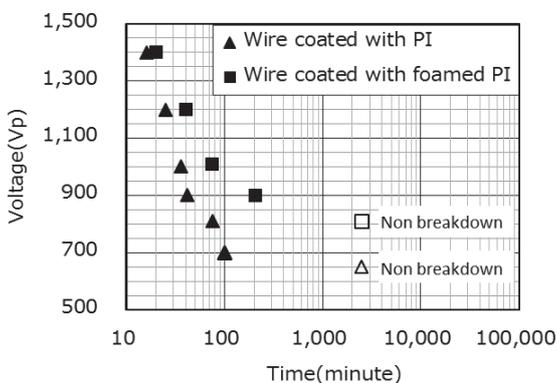
Fig. 11. Withstand Voltage Measurement Result (at 200°C)
