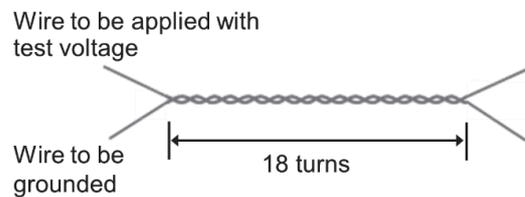
Fig. 5. Schematic Illustration of Twisted Wire Pair
