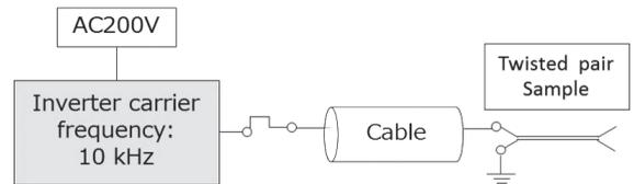
Fig. 9. Schematic Illustration of Withstand Voltage Life Measuring Equipment
