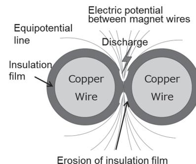
Fig. 2. Partial Discharge from Magnet Wire and Erosion of Insulation Film
