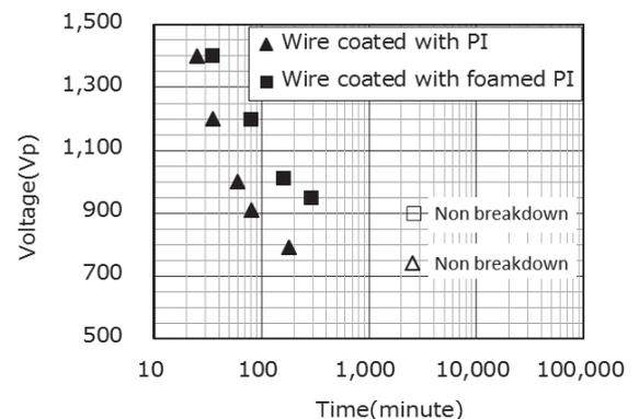
Fig. 10. Withstand Voltage Measurement Result (at 25°C)
