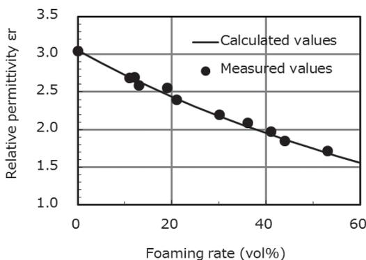
Fig. 4. Relative Permittivity of Foamed Magnet Wire
