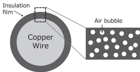
Fig. 3. Schematic Illustration of Foamed Magnet Wire
