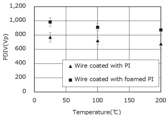
Fig. 8. High-temperature PDIV Measurement Result for Magnet Wire Coated with Foamed PI
