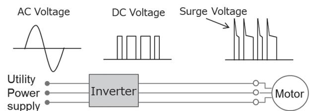
Fig. 1. Schematic Illustration of Inverter Surge Voltage
