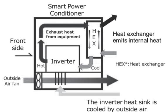
Fig. 4. Hybrid cooling
