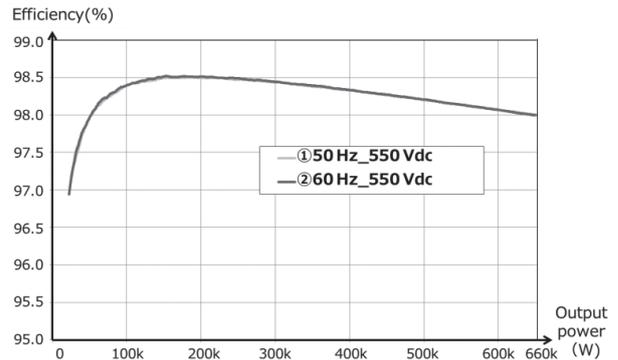
Fig. 3. Efficiency characteristics (at 550 VDC)
