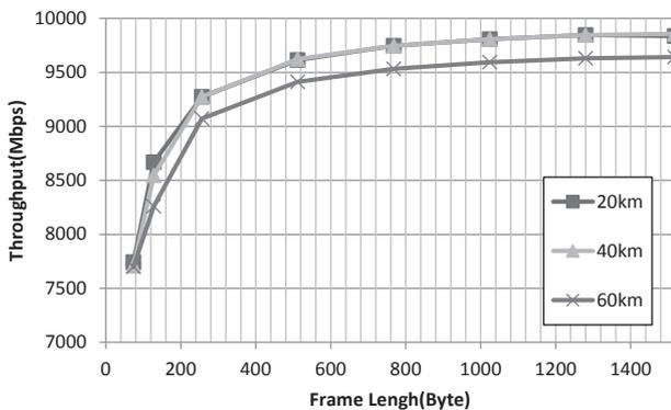
Fig. 3. L2 throughput with a connected 10G repeater
