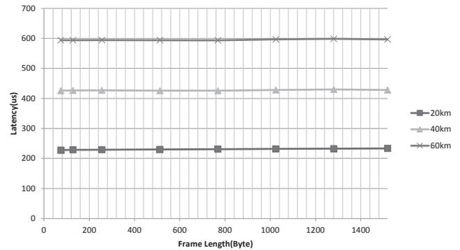
Fig. 4. Latency with a 10G repeater
