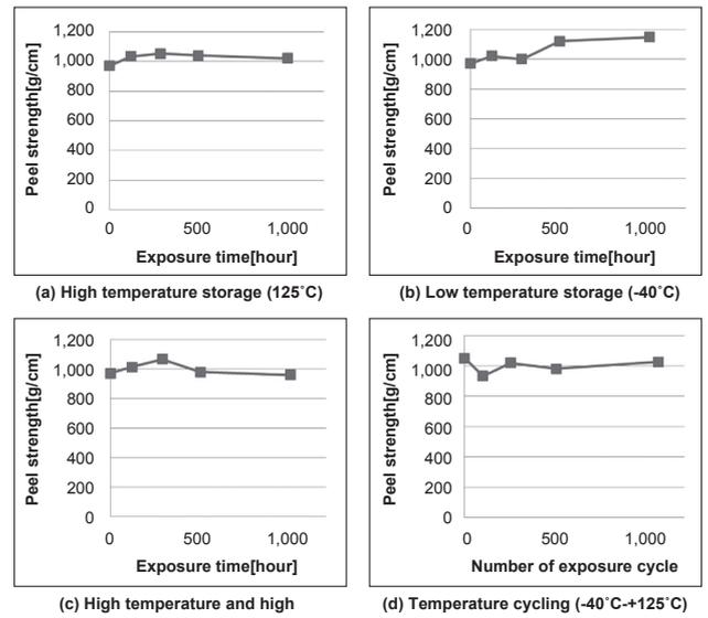
Fig. 4. Reliability for the peel strength of thermal resin
