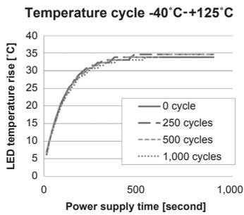
**Fig. 5.** The reliability of the cooling performance of new heat diffusion structure for temperature cycling test
