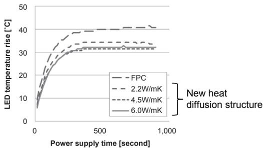
Fig. 2. Experimental result of the cooling performance
