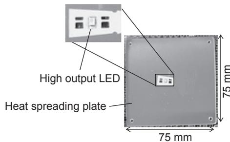
**Photo 5.** Test module to evaluate the cooling performance for the high output LED
