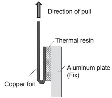
Fig. 3. Test piece and measuring method
