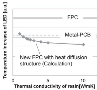
Fig. 1. Calculation result of the new heat diffusion structure
